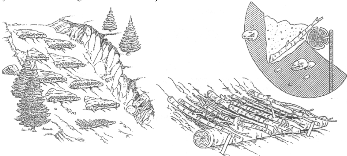
Figure 7. Modified brush layers can be built with either a log or a board for support. They should be staggered across a slope so that material rolling down the slope doesn't have a chance to get going before it is caught. The detail shows a modified brush layer prior to backfilling, while the section shows the normal backfill which creates a bit of a bench.
